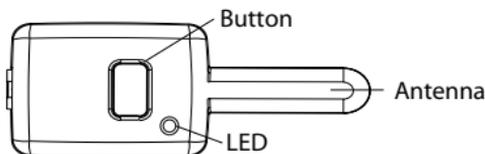
The Control Center, typically located on the upper part of the front windshield receives commands from your system. It consists of:
