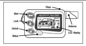
When used with a **4204**, immediately after a command is sent, the remote control switches to receive mode for 5 seconds while waiting for a confirmation signal. The only exception is for the Start command. The remote will always stay in receive mode, waiting for engine shut down feed back from the car.
